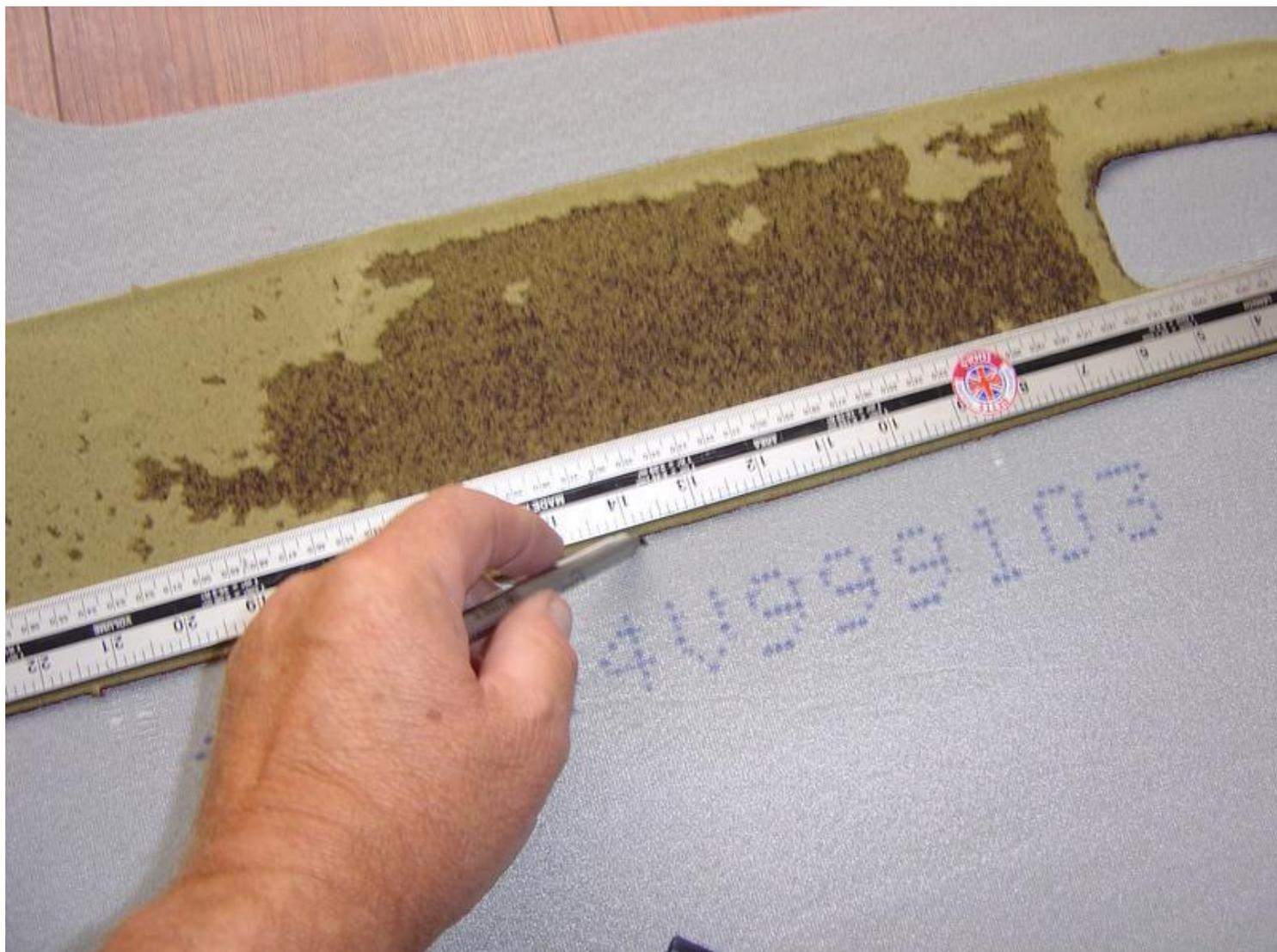
**CUT THE EDGES AS ACCURATE AS POSSIBLE BUT LEAVE ABOUT 2MM SPARE ROUND THE DOOR HANDLE**
