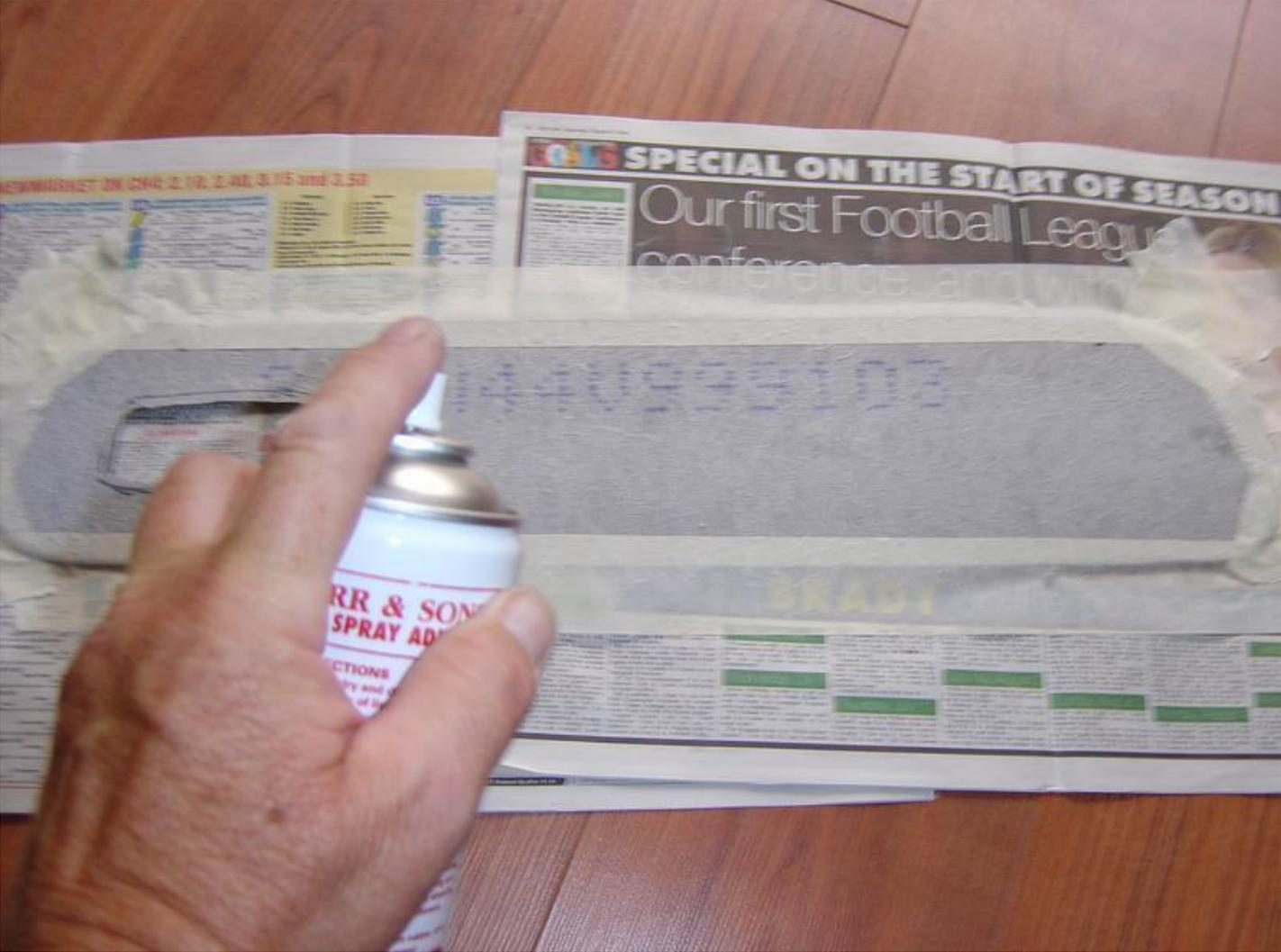
Leave for ten minutes and place in position, there is no need to spray the door card itself as the sticky material left after cleaning is still usable and you can reposition to get the right fit without any bother
