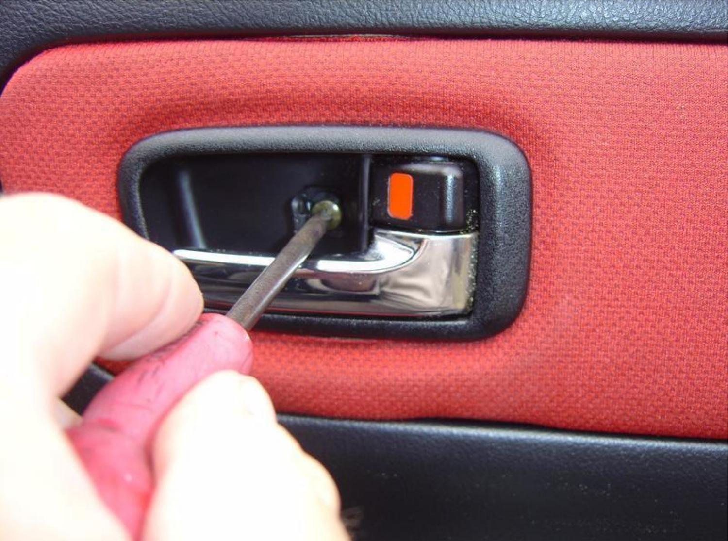
**PLACE FLAT SCREWDRIVER HERE AND GENTLY LEVER UPWARDS WHILE PUSHING WITH FINGER**
