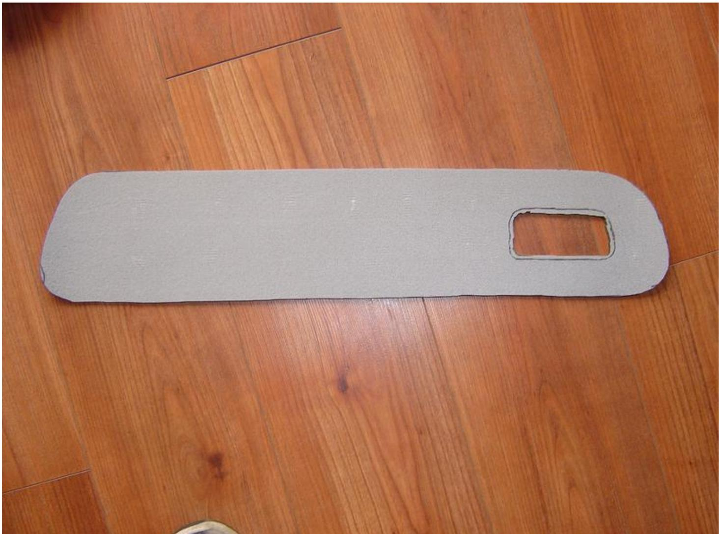
[MASK THE EDGE OFF BY ABOUT 10MM \(No adhesive needed here\)](#)
