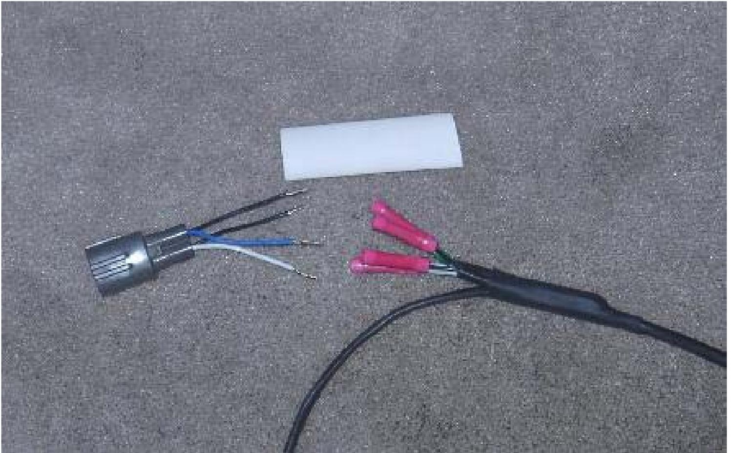
Attach connectors and O2 sensor to the wiring harness, in **the positions shown above**, using a crimping tool.
