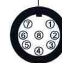
8 pins Binder 712 female connector external view
