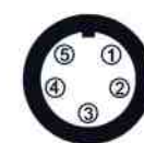
5 pins Binder 712 female connector external view
